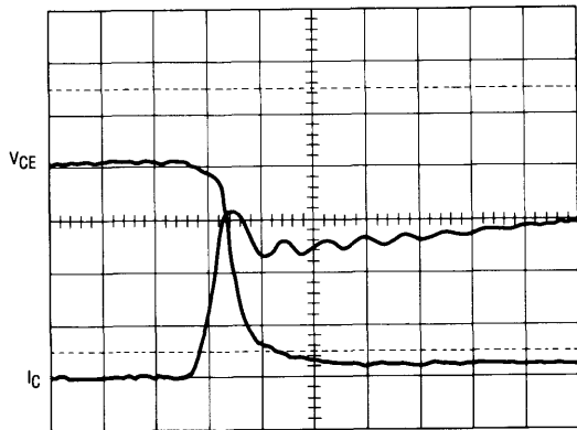
Figure 10b. Turn-on with an ideal diode (zener clamp). Test circuit as in Figure 16.
